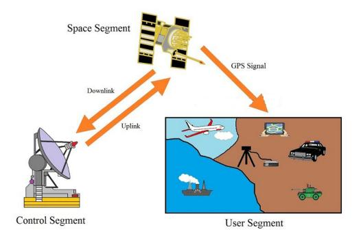
• **Working principle** - The tracker uses a process called <u>trilateration</u> which uses the position of 3 or more satellites from GPS satellites and its distance from them to determine latitude, longitude, elevation, and time.
